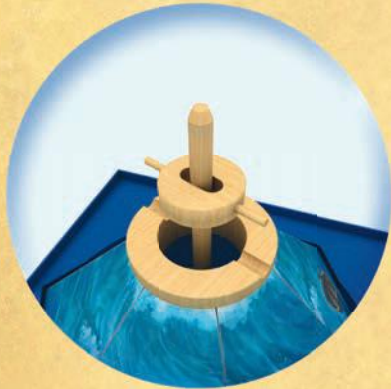
C. Place the joint of the ball-bar on the wooden ring in such a way that the ball sinks into the hole and the two retaining rods come to lie in the troughs of the ring.
